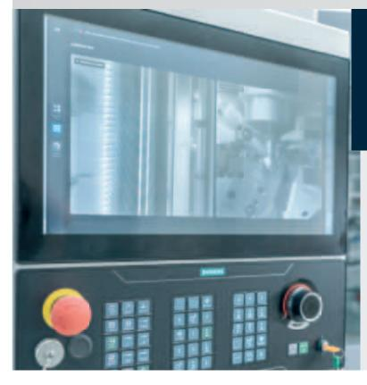
» Camera image of the machine room on the panel: The operator can check here, for example, whether the chip formation is causing a fault in the process.
