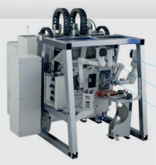
**Robot 3:** Parts handling from the transfer station to the outside
