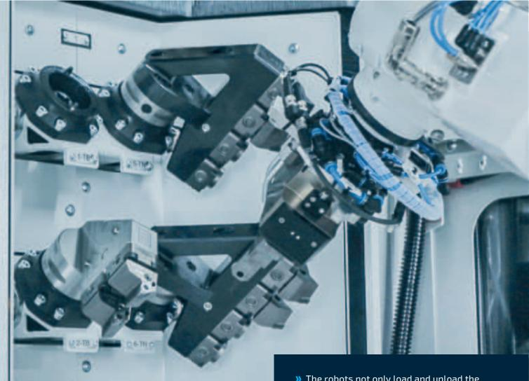
» The robots not only load and unload the machine (pictured here), but also change the tools.
