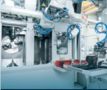
» View of the robot loading of the VST 50: While R1 and R2 load and unload the machine, R3 takes care of the transport between the loading station and the outer conveyor belt in the back ground.
