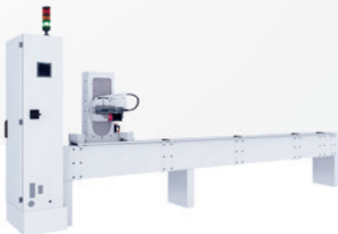
EMAG TrackMotion simplifies linking multiple machines.
