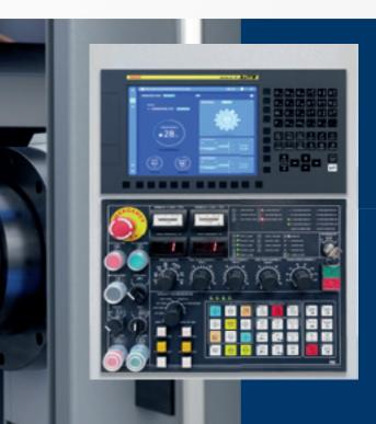
The latest generation of Fanuc 0i TF Plus control offers extensive possibilities for process optimization. While machining is in progress, programs that follow can be created or optimized. Standardized interfaces make it easy to integrate the machine into existing production lines.
