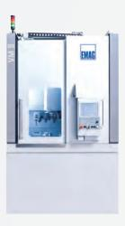
The vertical turning centers in the VM Series are designed for the highly productive manufacturing of workpiece families with a wide range of parts. A tool turret with twelve tool positions, depending on the required tool interface in a BMT or VDI version, is available for machining. The turret can be equipped with driven tools to carry out drilling operations, for example.
