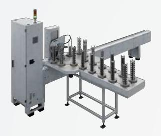
TrackMotion is a linking system to connect two or more VL/VLC or VT/VTC machines and additional components such as feeding and discharge belts, measuring equipment, etc. The TransLift lift and turn-over unit runs on a modular rail system and features a programmable electric gripper which can transport and turn workpieces.
