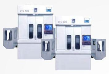
The strength of the VTC Series machines is their 4-axis machining of large quantities of shafts up to 400 mm in length. Since the machine concept comprises a fully integrated automated loading and unloading system, a manufacturing system can be created, which features very short transport distances. The machines are loaded and unloaded by the two turrets, which ensures that the process is fast and straightforward.
