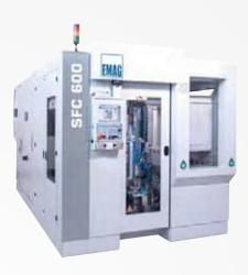
The joining machine SFC 600 features our patented thermal stress-free joining process combining precision and high flexibility for the heat shrinking of components (cams, bearing rings, sensor wheels, etc.) onto camshafts.
