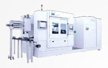
EMAG's ELC 160 HP is a system that has been specially developed to meet the requirements of transmission production. Our consistent striving for maximum productivity in large-scale production by drastically reducing cycle times makes this machine one of the most efficient laser welding systems on the market.
