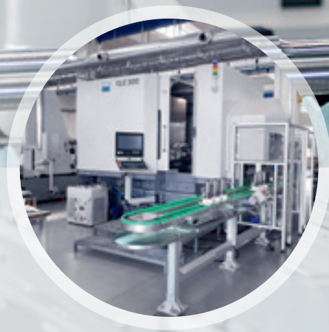
Stacker cell with surrounding conveyor belt.
