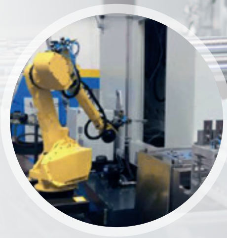
Robot loading from the rear with loading door.
