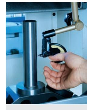
The EMAG Geometry-Set is used for regular and preventative inspection as well as the retrieval of tool carrier geometry following a collision or tool breakage. This provides protection against a decrease in quality and consequential damage.
