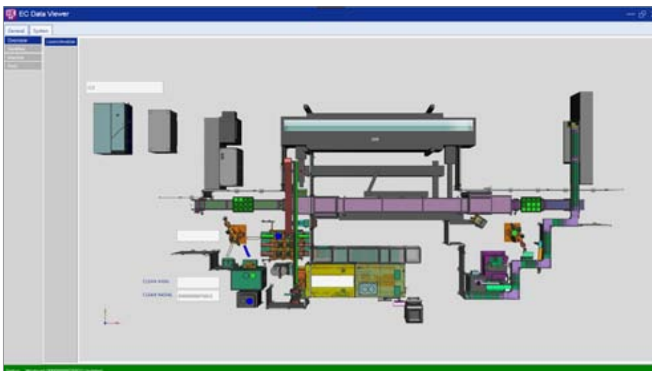
Layout of a manufacturing system, including visualization of parts flow and of production status
