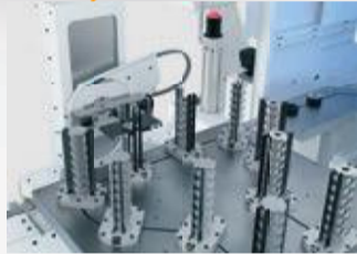
Parts storage area for up to 400 workpieces, including TrackMotion
