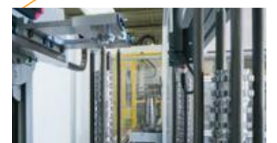
Parts storage area for a maximum of 400 workpieces, including TrackMotion
