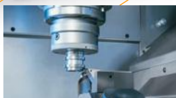
Turning of the second side (OP 20)
