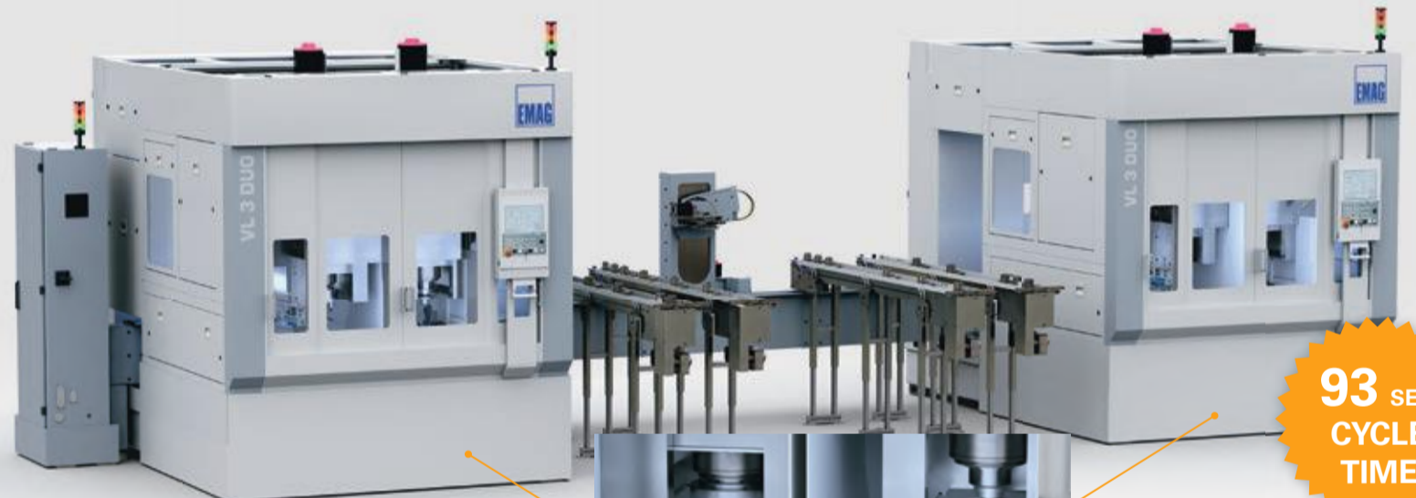
Parts storage area for up to 400 workpieces, including TrackMotion
