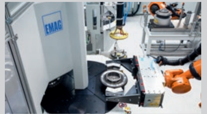
The housing parts and the ring gear are cleaned on the newly developed EMAG laser cleaning machine before being welded.
