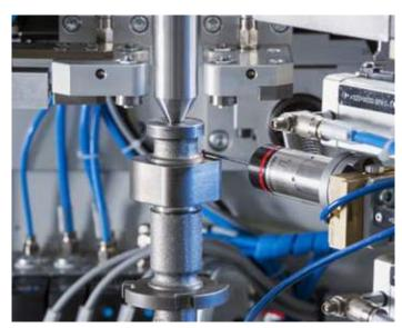
**Quality inspection of joining results:** The probe tests the axial position of the workpiece after the joining process. The prescribed slump is automatically corrected in the case of deviations.
