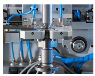
**Joining process:** The pump cam is in the cooling phase at this position. All workpieces are gripped with roll grabs. This ensures maximum thermal insulation, in order to minimize loss of heat energy.
