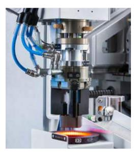
**Workpiece recognition** using dot patterns or Data Matrix Code (DMC) for workpiece identification and determining the correct workpiece position. The piece is then transferred to the induction heating station.
