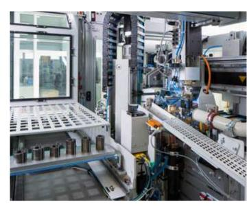
**Joining parts** (cams, sensor wheels, other parts) are supplied on two interchangeable pallets based on position. While the workpieces from the first pallet are automatically removed via a loading portal, the second pallet is already being loaded up.
