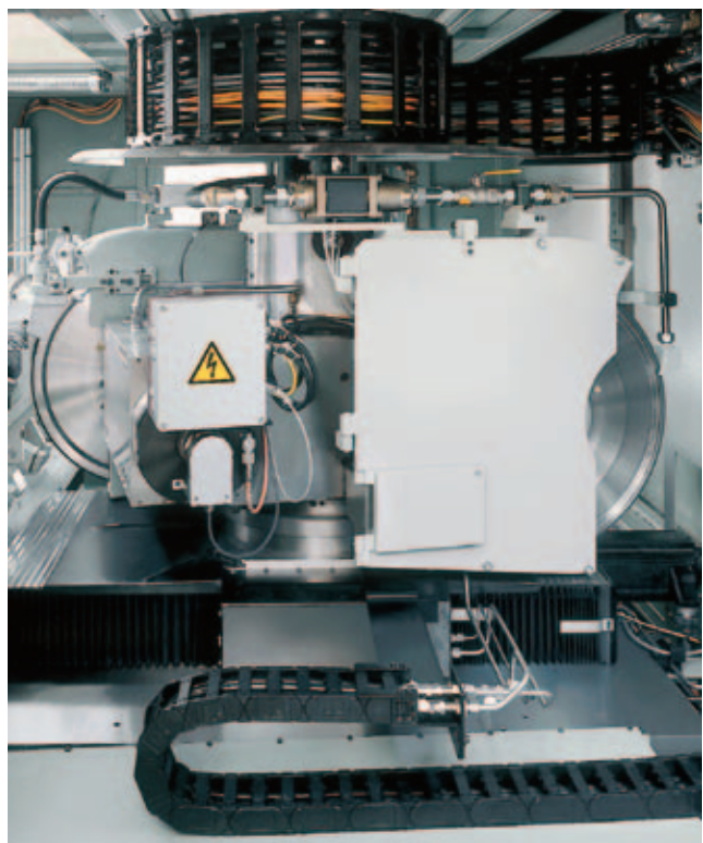
Flexible CBN grinder with B-axis.
