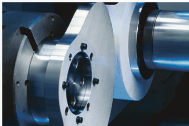
Grinding a radial cam for textile machines
