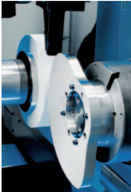
SK 204 machining area Grinding a radial cam
