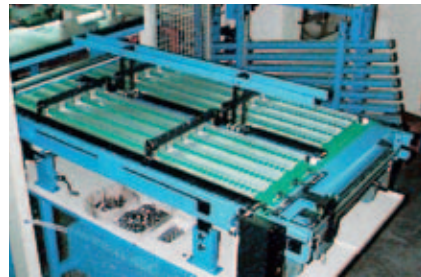
Long-time recirculating storage conveyor
