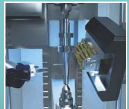
Hobbing, radial drilling, deburring, turning
