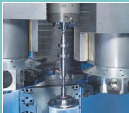
4-axis turning, milling and drilling operations with driven tools
