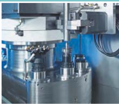
Cutting to length + centering, deep-hole drilling, milling, thread cutting, axial milling, slot-milling
